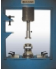
COMPRESSION ON CEMENT TEST SPECIMEN
